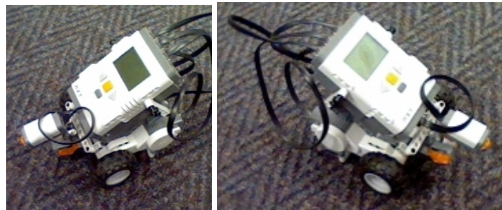
Figure 4.4: The modified Tribot design used in the project
