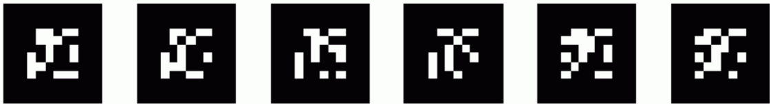
Figure 4.6: Five Enumerated Markers Used in the ARToolKit+, each is associated with a market ID in the ARToolKit+.
