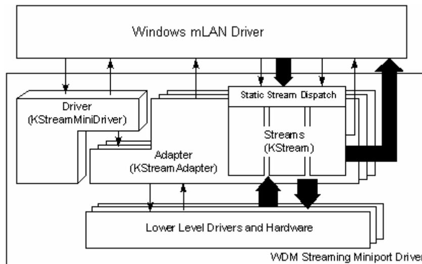
**Figure 6.4: Kernel Streaming Architecture**
